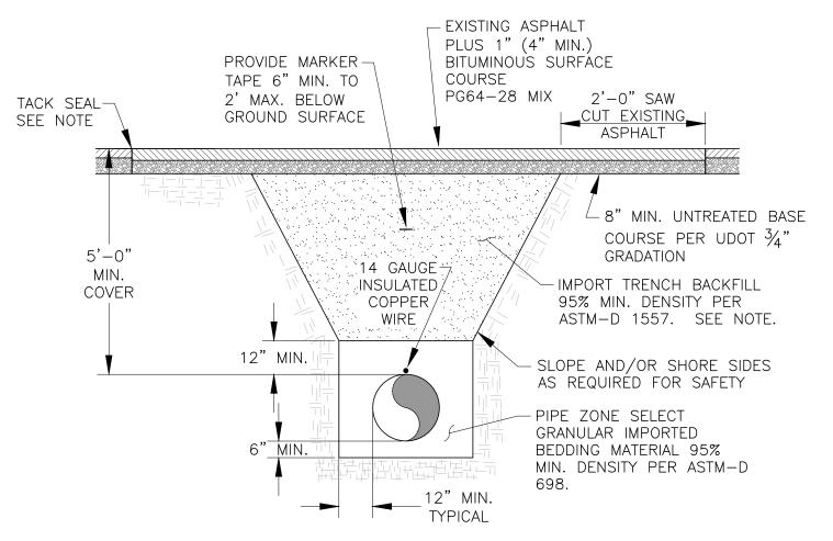
NOTE: REMOVE EXISTING TRENCH BACKFILL AND REPLACE WITH A1-a (3" MINUS) MATERIAL. COMPACT IN 8-INCH LIFTS.
